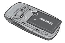
2. Press down until the battery snaps into place.
